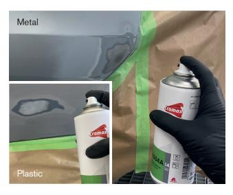
The new PS1504A Quickfill Primer-Surfacer offers improvements in productivity particularly where smaller repairs are concerned. The repair process is shortened considerably thanks to a reduction in process steps, simple universal application, and rapid-drying performance.
